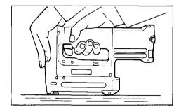
If the tool becomes jammed, do as follows. First, remove the battery cartridge. Open the sub-magazine and remove the stuck staple using a screwdriver or the like.
